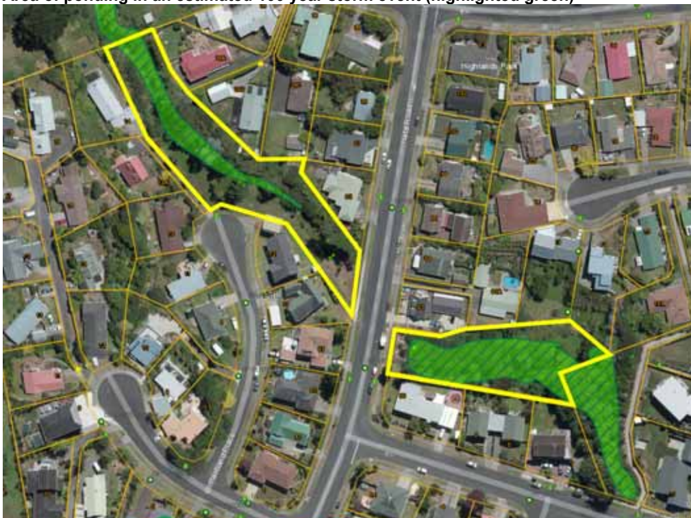
Area of ponding in an estimated 100 year storm event (highlighted green)
